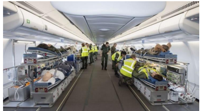
A French Air Force Morphée A330 Airbus flew patients from Basel-Mulhouse airport to Marseilles. The plane is specially configured as a long-haul intensive care unit.
